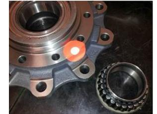
4. Flip the hub and use the same procedure to remove the second bearing cone and seal.
