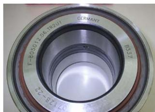
**Bearing oil side.** There isn't any place to fit the o-ring.
