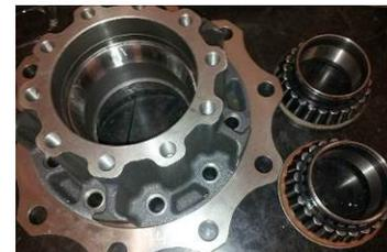
5. To remove the two outer bearing cups from the hub, use a hydraulic press and a proper pushing tool (see drawing below).
