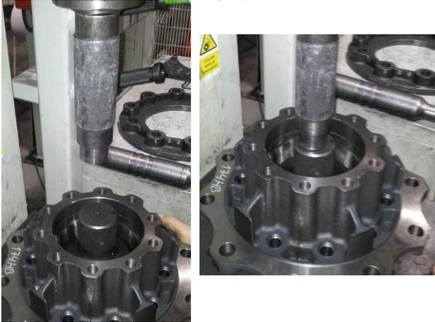
**IMPORTANT:** check the force exerted by the press to remove the bearing cup. If the force is lower than 10kN [1ton=1000kgf], the hub can NOT be reused, it must be discarded and replaced by a new complete hub & bearing assembly.
