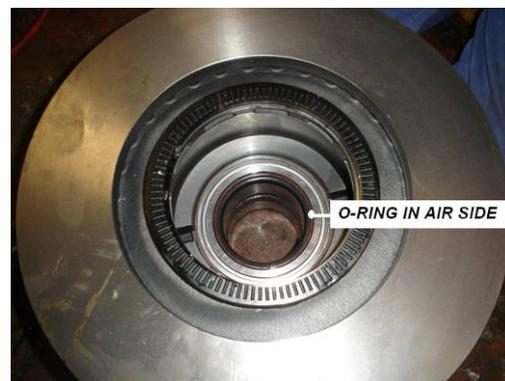
**CAUTION:** In spares the o-ring can be provided as separate component to be assembled on the bearing groove or already assembled in the bearing groove.
