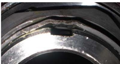
**CAUTION:** bend out the staked area of the nut fully so as not to damage the threads when removing the nut. Also care should be taken not to drive the tool in deeper than the staked area of the nut as this could damage the threads of the nut or the spindle.
